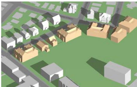
Project Analysis: Computer model shows cast shadows of proposed buildings at noon, December 22.
